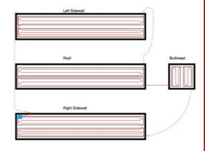
In the general construction, SatSENS.loop-wall basically consists of two GRP (Glass Reinforced Plastic) strips with integrated cables that are glued to the side wall. The roof and the partition wall are also protected by two bonded GRP strips.
