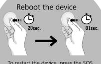
To restart the device, press the SOS button for 20 seconds then stop, then press briefly for 1 second.
